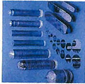
A substrate made of Gallium Arsenide or Indium Phosphide
